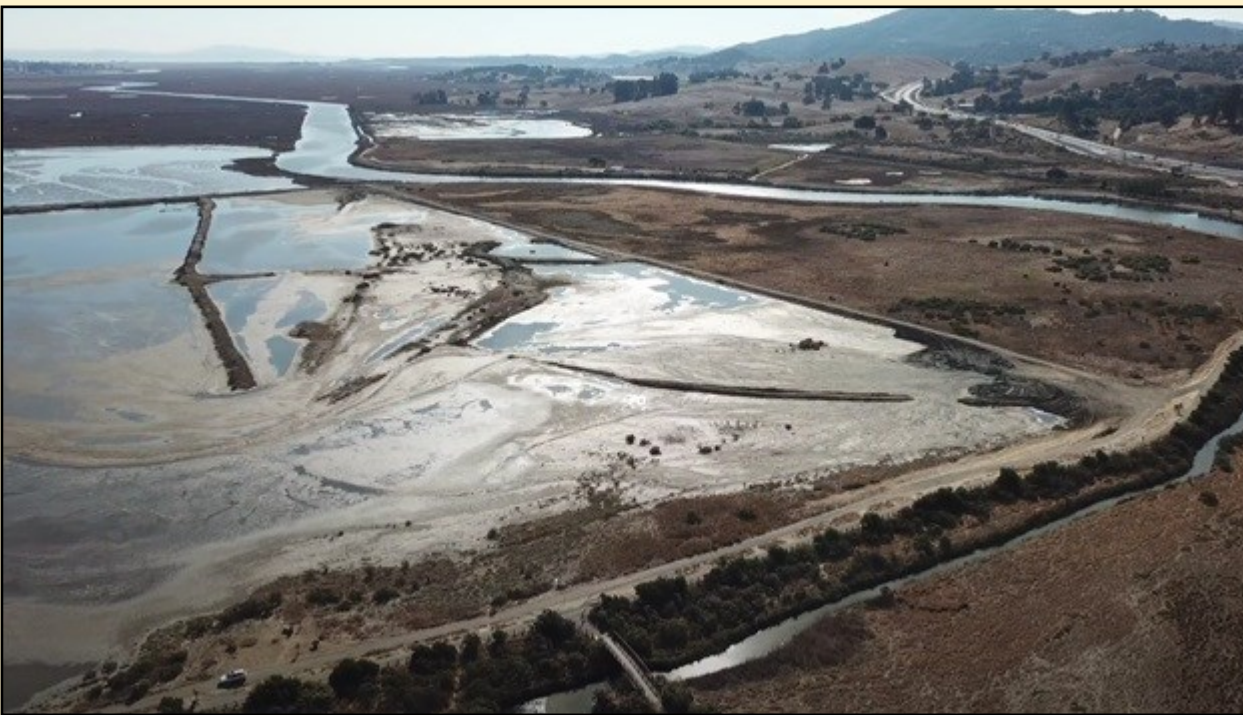
Fig.: Dredge Spoils are deposited on the western side of the Central Pond. Dikes channel and slow the flow.
