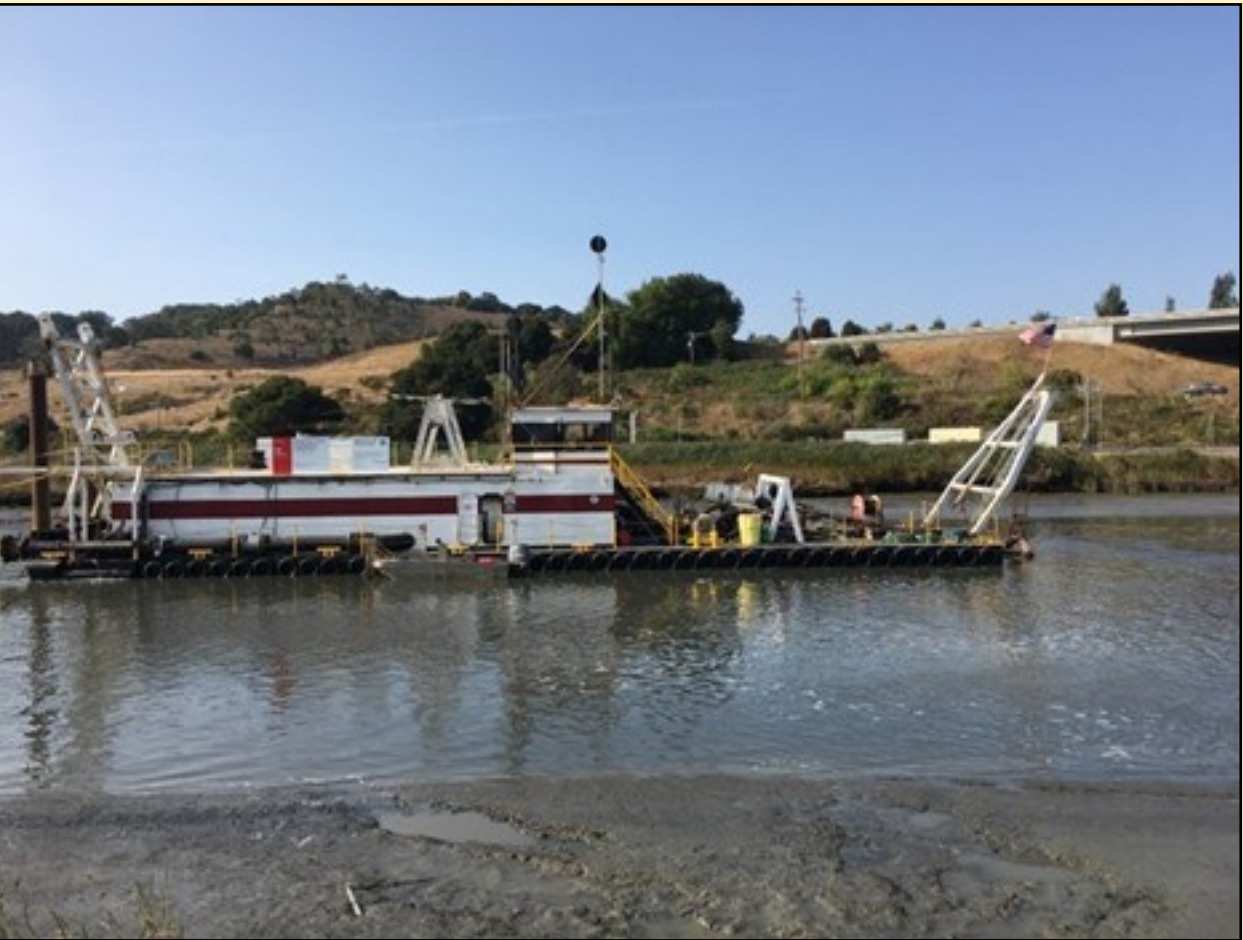
Fig.: Cutter Suction Dredger working near 101 overpass.
