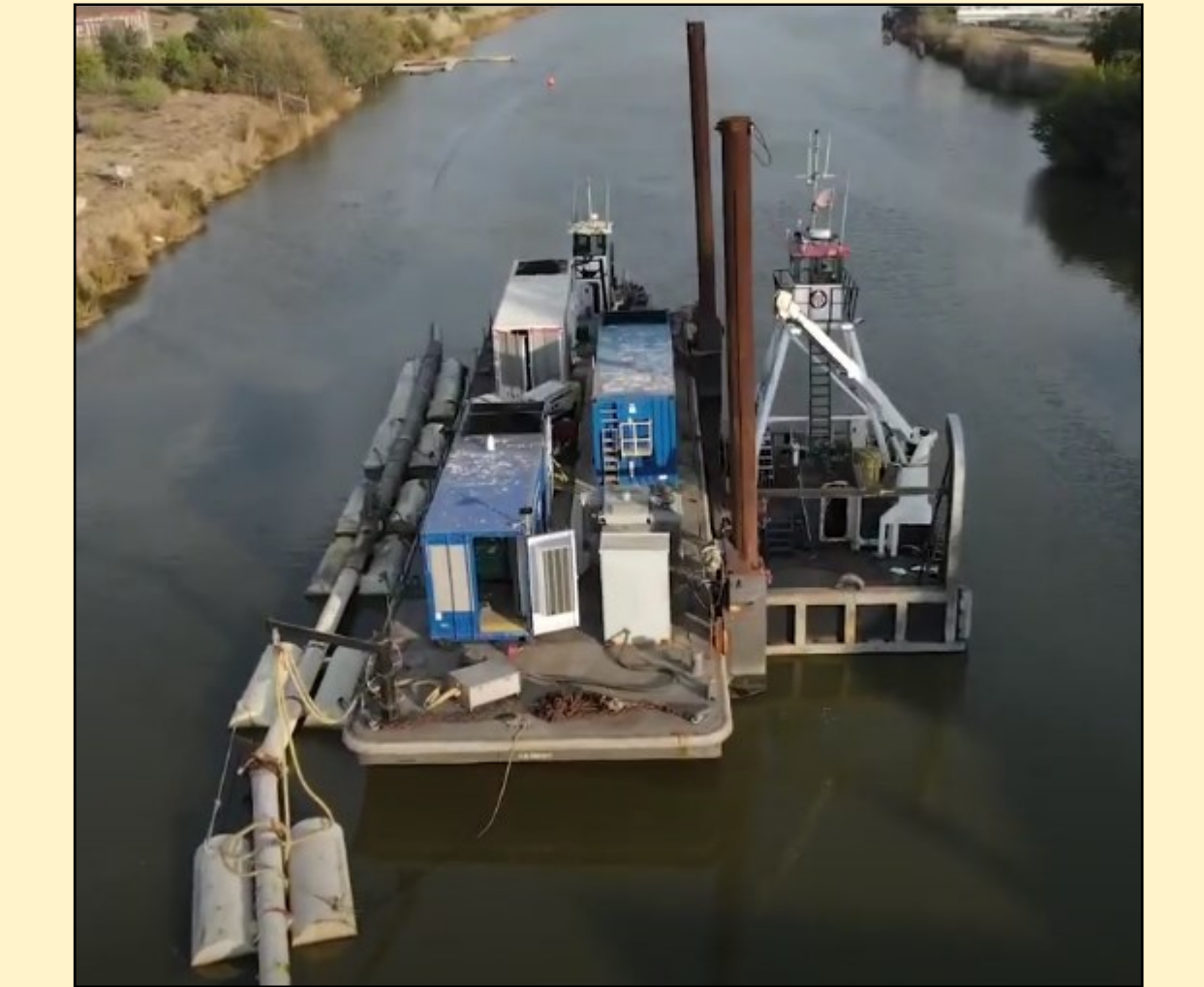
Fig.: The support barge is layered with electrical generators, pumps, and extra equipment to help move the dredge spoils down the large rubber tube to Shollenberger Park Central Pond. Other smaller support boats help move crew and keep any water traffic from crossing over the pipeline.
